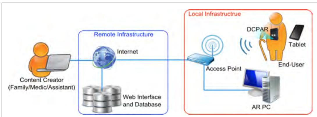
Figure 2. Design of the experimental Assisted Living system.
